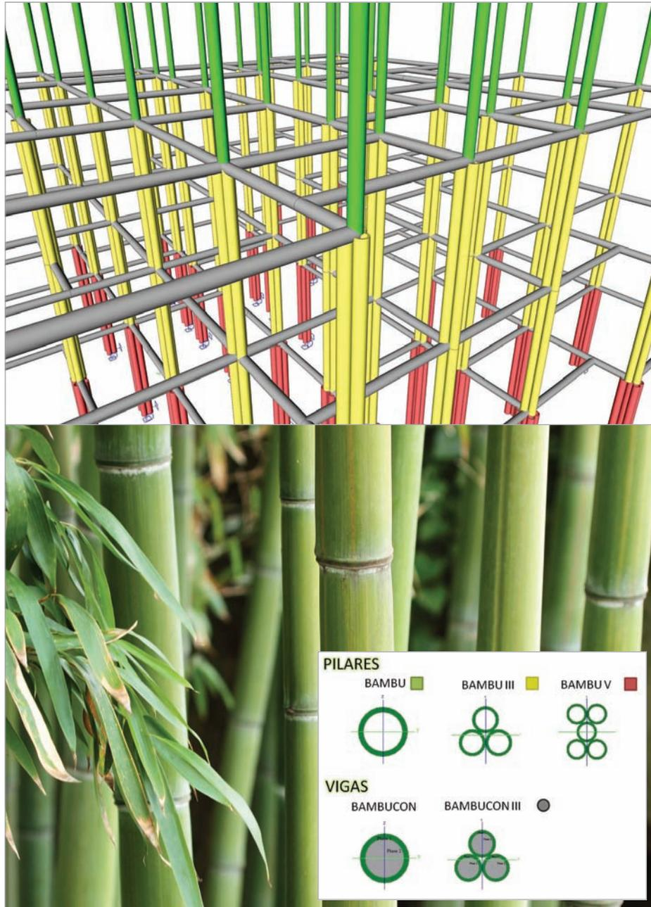
With the aim of ensuring environmental sustainability in construction, a mixed material was developed, composed of bamboo and filled with concrete, combining the advantages of both materials in a single element.
