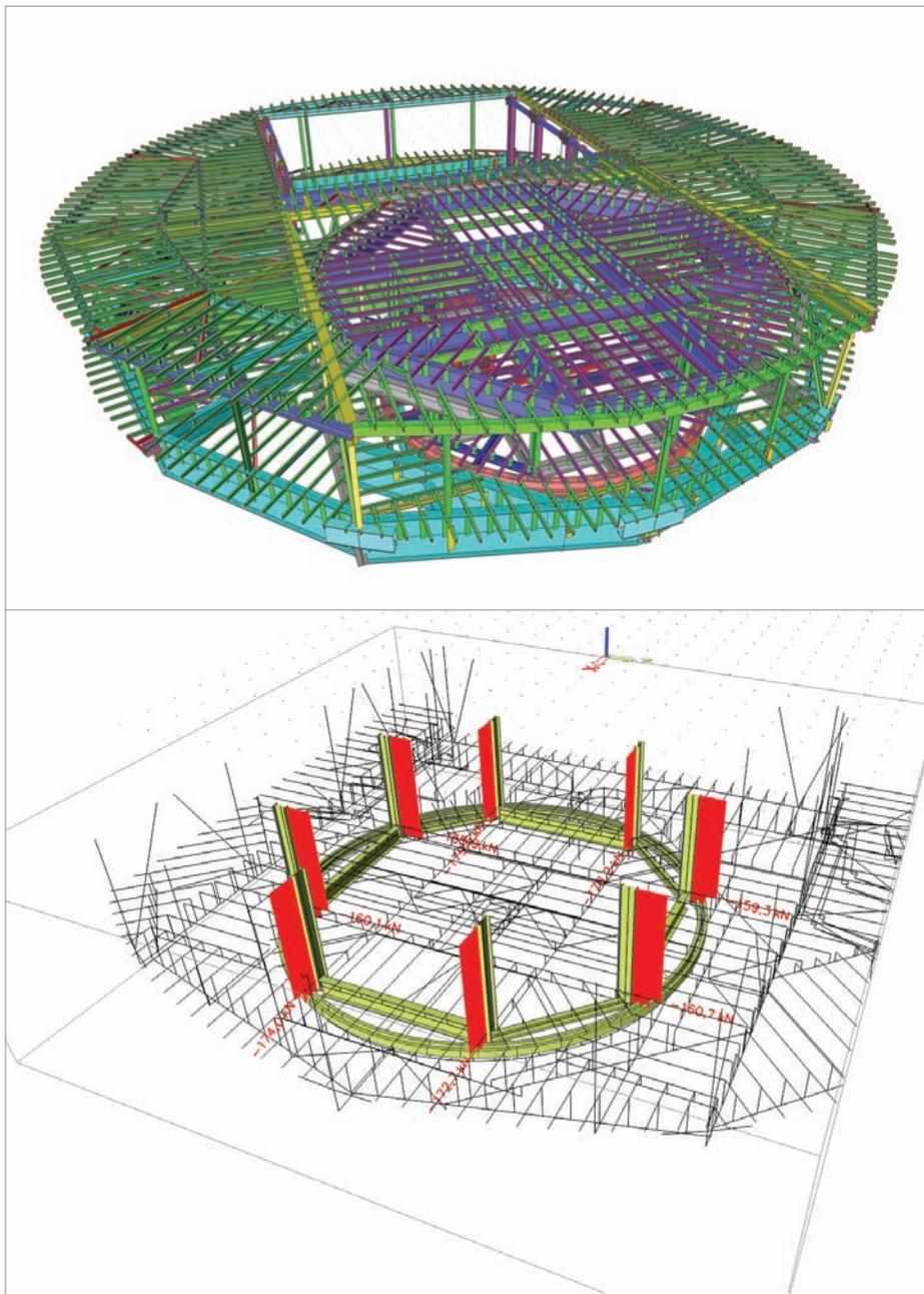
The revolving stage in the new Music Theatre Linz is a two-storey steel construction with an outer diameter of 32 m. The height of the two storeys is 3.95 m and is adapted to the surrounding building. The space underneath the revolving stage is used as an underground parking garage.
