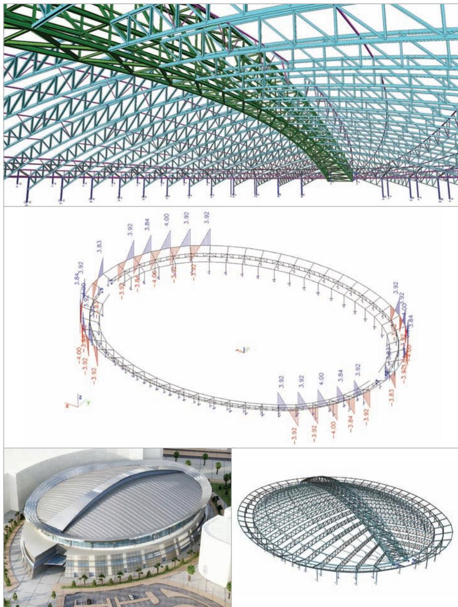
The arena roof is part of the King Saud University Sport Campus in Riyadh (Saudi Arabia) and it is the main feature of the sport campus. The building is for indoor athletics and also has the ability to hold conferences. The basic form of this building consists of a large single span roof with a central arch truss supporting secondary trusses. The steel structure covers an independently stabilised reinforced concrete frame.
